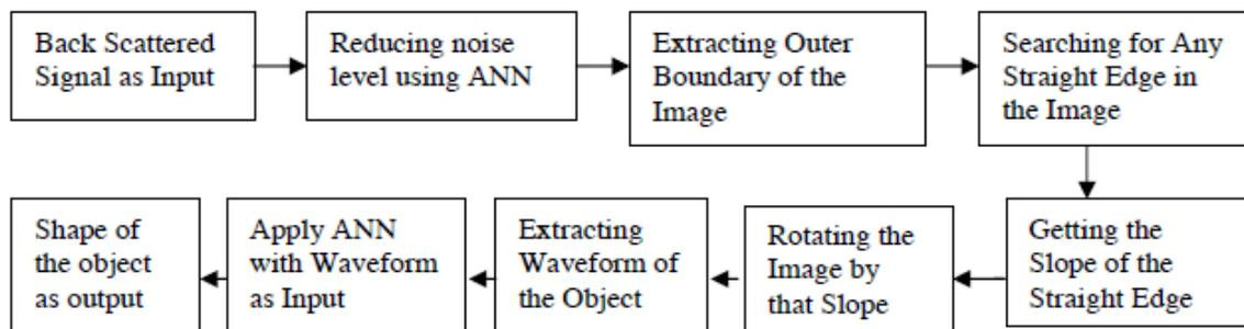
**Fig 6.** Block diagram of the system recognizing the shape of the buried object when orientation effect has neutralized.
