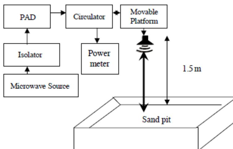
**Fig 1.** Schematic diagram of monostatic scatterometer.
