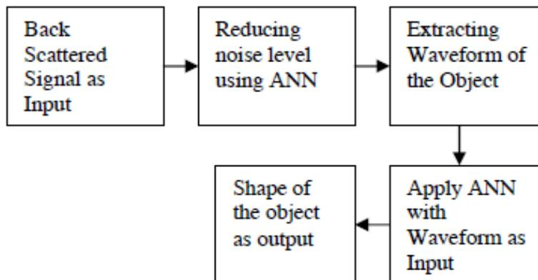
Fig 4. Block diagram of the system for recognizing the shape of the metallic shallow buried object without consideration of orientation effect.
